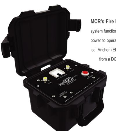
MCR's Fire Panel Filter provides filtered DC power to ensure firing system functionality when used with inferior firing systems and clean DC power to operate electronic equipment such as MCR's Electro-Mechanical Anchor (EMA). Each Fire Panel Filter (FPF) reduces "dirty" output from a DC source and filters the ripple. The FPF has a maximum operating voltage of 500V with a 5 Amp fuse limitation.
